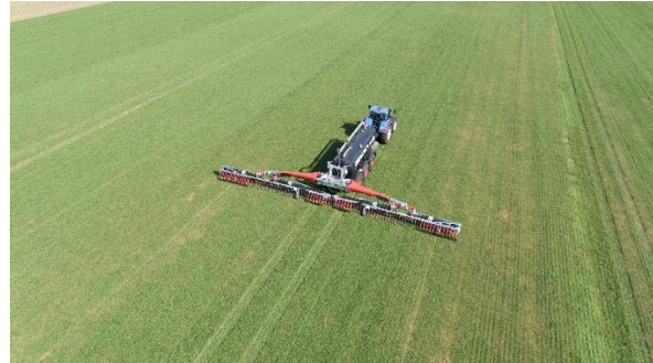
Image 2: The new BlackBird (here in a working width of 21 meters). The flexible trailing shoe linkage allows working widths of 30, 27, 24 and 21 meters without any overhang to the selected width.
