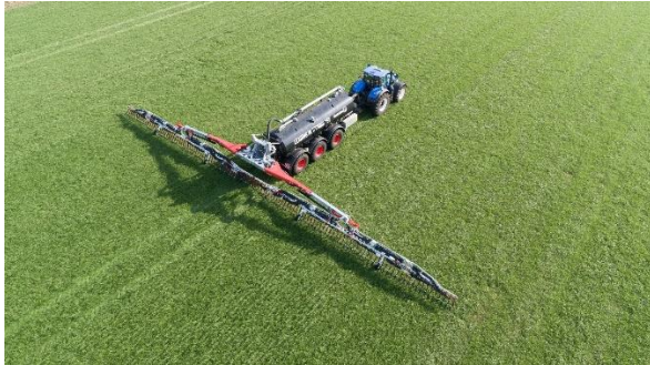
Image 1: The new Vogelsang trailing shoe linkage BlackBird in a working width of 30 meters.
