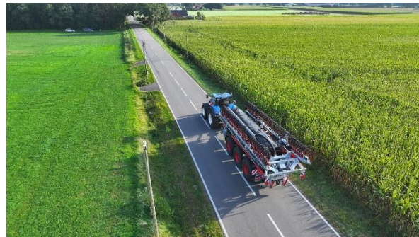
Image 4: With an arm length of 9 meters in transport position (measured from the lower link), the new large BlackBird can be attached to a wide range of liquid manure tankers.
